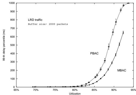
Fig. 6. Delay performance vs link utilization, using a 2000 packets buffer
